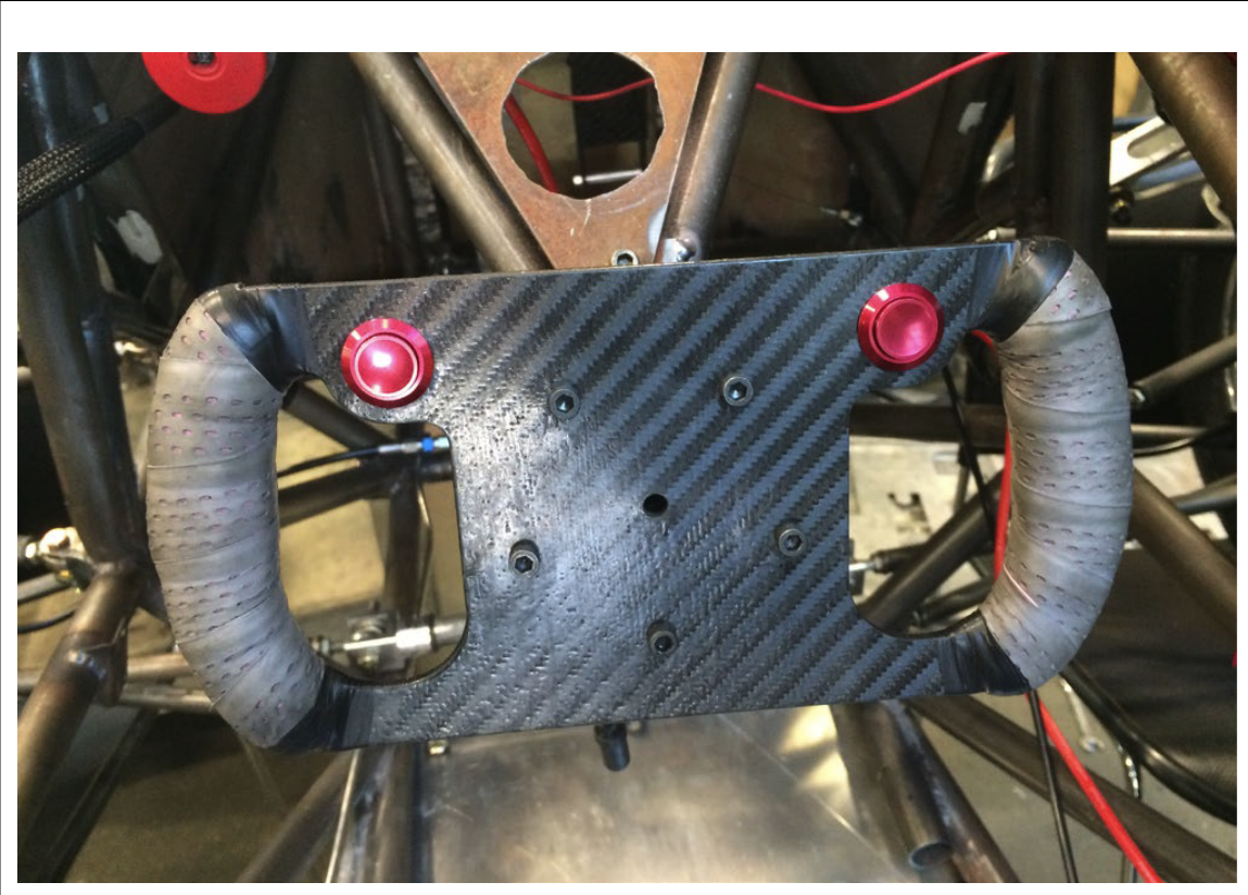
Figure 7: Finished steering wheel with buttons for shifting.
